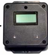
Wireless Transmitter at Entrance
